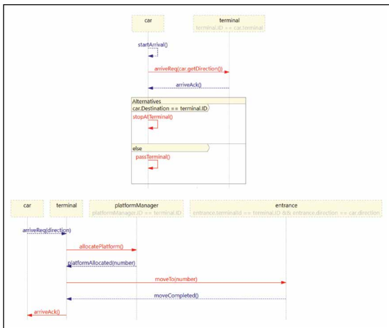
Figure 10. Top LSC: Car arrival at a terminal. The car first calls startArrival . It then sends an arriveReq message to that terminal and waits for acknowledgment. Depending on whether the next terminal is its destination or not, it stops or passes through. Bottom LSC: Arrival request. The terminal asks the platform manager to allocate a platform and waits for an approval containing the allocated platform's number. Then the car is sent to the corresponding entrance. Note in both LSCs the symbolic lifelines, which are concretized (instantiated) to specific objects via a binding expression; for example, in the top LSC, the car's terminal property is compared with the ids of all terminals.
